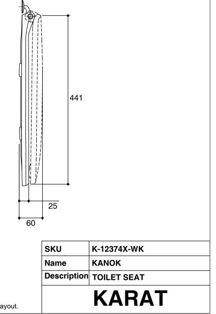
\* The recommended dimension for installation can be adjusted according to user preferences and layout.
